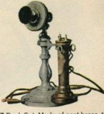
1897 Desk Set. Made of cast brass, this ancestor of the upright desk set represented a refinement of earlier models.
