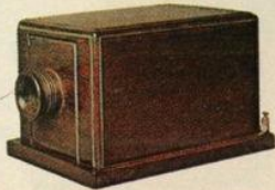
1877 First Commercial Telephone. The round, camera-like opening served as both the transmitter and the receiver.
